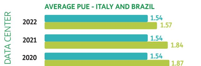
**Power Usage Efficiency (PUE)** relates the energy consumed by IT equipment to the energy consumed by the entire data center. The closer the value is to 1, the more efficient the data center is because it directs energy only to the IT portion. The industry average is 1.55.
