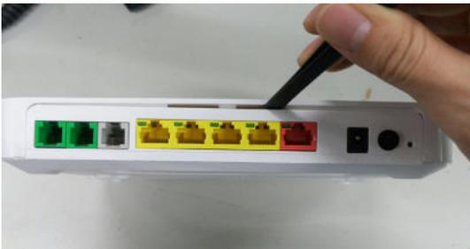
(4) Rotate the housing to separate Top cover and bottom cover
